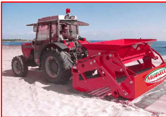
Upper tank hydraulic discharger
